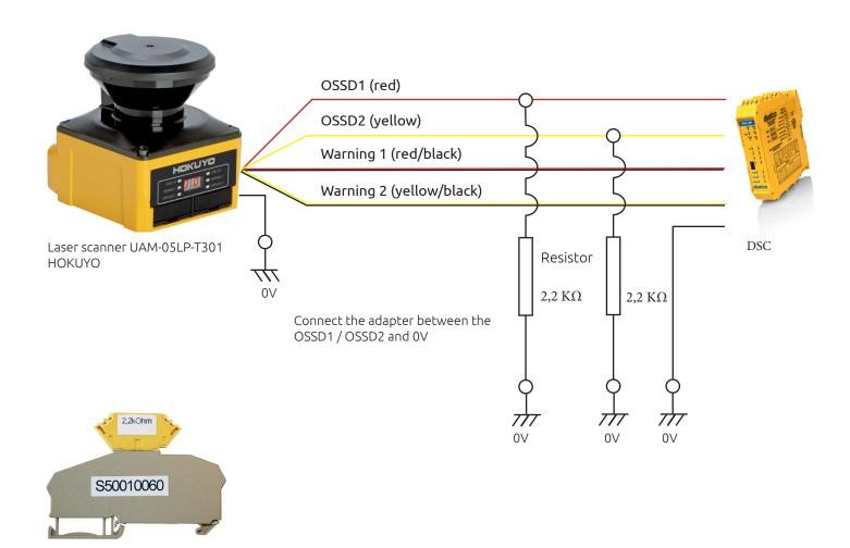
CONTA-CLIP resistor 2,2 kOhm Art.nro. S50010060 contains 2 resistor
