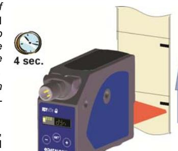
If the detection has been successful, the sensor returns to normal functioning. If it fails due to insufficient contrast, the 'Lo' test blinks on the display. Press the SET push-button to repeat procedure until releasing the button (the 'dYn' text blinks on the display). The sensor returns to the previous setting by pressing + or -.
