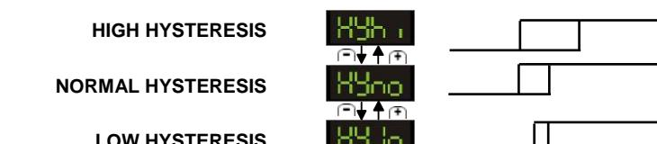
The level switches by pressing + or -.
