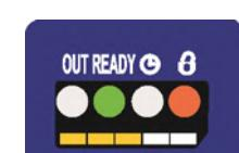
Increasing or decreasing the threshold, the right or left LEDs blink with a frequency proportional to the difference from the initial threshold value.
