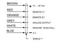
\* = Connect the unused REMOTE wires to 0 V.
