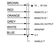
\* = Connect the unused REMOTE wires to 0 V.
