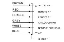
\* = Connect the unused REMOTE wires to 0 V.
