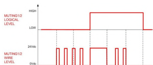
Figure 31 - Muting filter enabled
