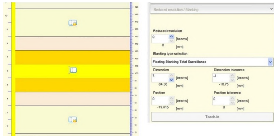
Figure 60 - Floating Blanking with total surveillance
