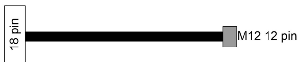
Figure 3 - Pigtail cable Blanking configuration for receiver (CS-G1-70-B-002)
