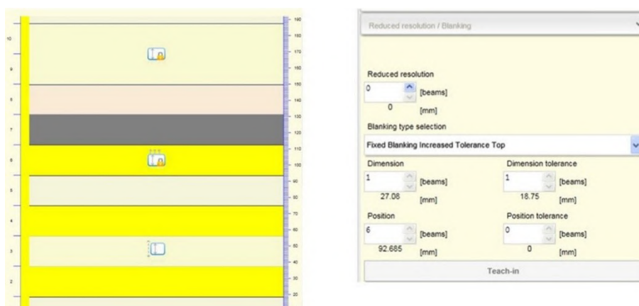
Figure 59 - Fixed Blanking with increase tolerance
