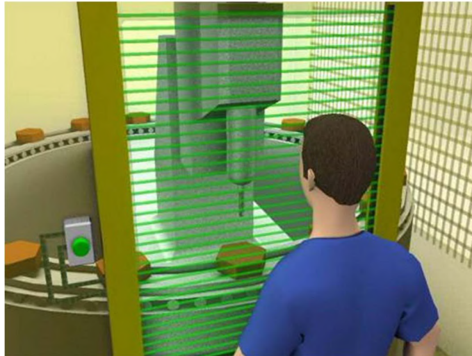
Fig 5 - Operating point protection on drilling machines
