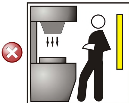
Fig 10 - Wrong light curtain positioning
