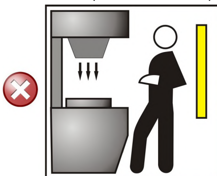
Fig 10 - Wrong light curtain positioning
