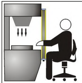
Fig. 8 Safety light curtain positioning
