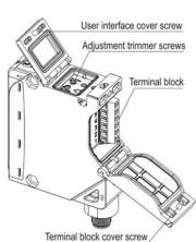
Tighten all screws surely to maintain the water-proof characteristics for IP67 (IFC/FN60529)
