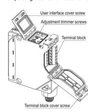
Tighten all screws surely to maintain the water-proof characteristics for IP67 (IEC/EN60529).
