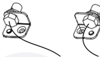
Figure 2.16 SMA Connector Installation
