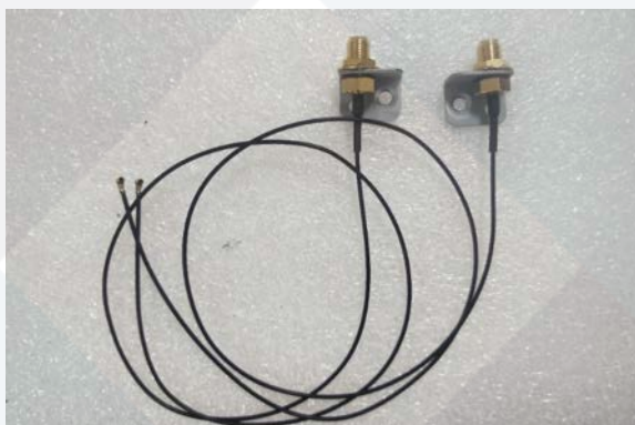
Figure 2.14 Assemble the Brackets to the Antenna Cables
