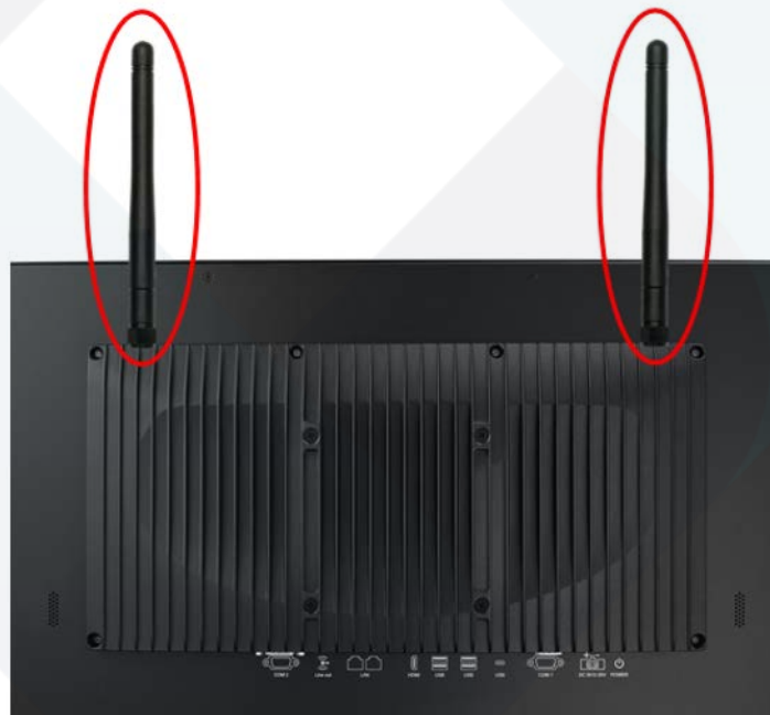
Figure 2.16 Attach the Wi-Fi Antennae
