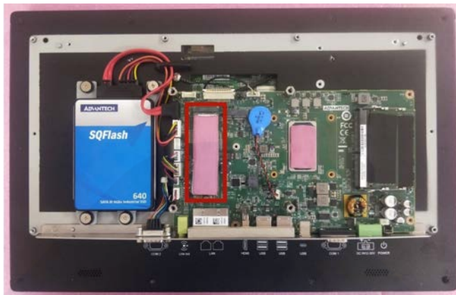
Figure 2.13 Affix the Thermal Pad to the M.2
