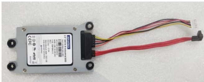
Figure 2.10 Secure the SATA SSD with Screws
