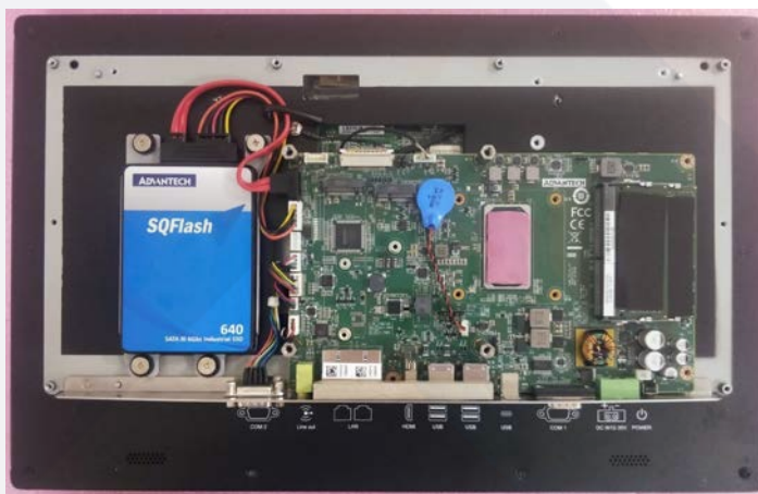
Figure 2.11 SATA SSD Connected to the Motherboard
