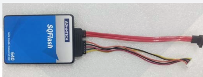
Figure 2.9 SATA Cable Connected to the SATA SSD
