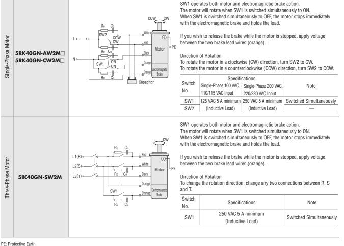
• R<sub>0</sub> and C<sub>0</sub> indicate surge suppressor circuit. [R<sub>0</sub>=5 $\sim$ 200  $\Omega$ , C<sub>0</sub>=0.1 $\sim$ 0.2  $\mu$ F, 200 WV (400 WV) ]
