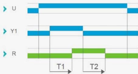
Function Ad: Delay on Start
