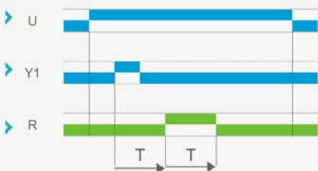
Function At: Summation Time Relay
