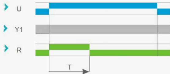
Function Ht: Interval with Memory
