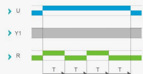
Function Di: Flasher (Symmetrical) - ON Start
