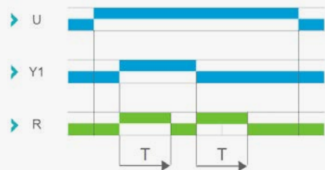
Function C: Off-Delay (Delay on brake)
