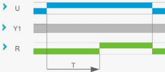
Function Ac: On/Off Delay (Delay on make/break)
