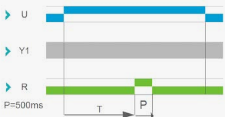
Function P: Pulse delayed relay
