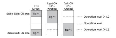
The Orange LED is an operation indicator. For Light On Type, it will light when the beam goes through. For Dark On Type, it will light when the beam is interrupted.
