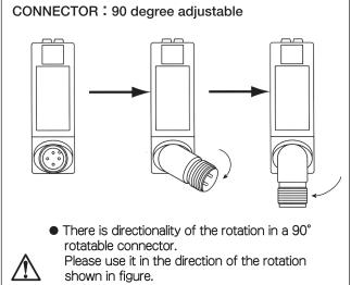
The connector might break for the wrong use in directions other than showing in figure.
