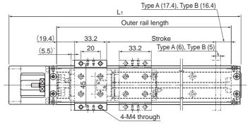
\* Distance between the mechanical stopper and the stroke starting position.
