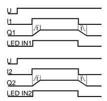
When triggering the input I1, the voltage on output Q1 will be raised to the nominal value linearly during the preset time slot. The motor is accelerated to full speed.
