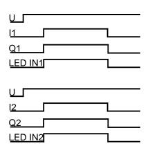
Triggering the input I1 switches on the output Q1 (e.g. electromagnet) immediately.
