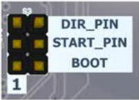
Fig. 5. START\_PIN and DIR\_PIN jumpers
