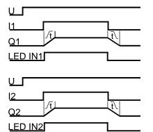
When triggering the input I1, the voltage on output Q1 will be raised to the nominal value linearly during the preset time slot. The motor is accelerated to defined speed.
