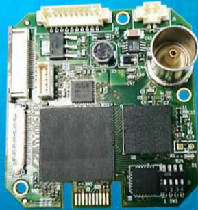
More than a video transmission module, the Twiga HD-SDI interface board for Tamron MP1010M-VC has been designed to be the heart of your industrial vision system.
