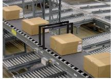
Two different models are available: high resolution (AS1-HR) or standard resolution (AS1-SR). In the first case the light array has 16 beams, while in the second case the beams are reduced to 6. In the AS1-HR model, the selection inputs of the SCAN MODE, can configure 4 different crossed-beam scanning modes. These different modes allow to vary the detection performances, in particular the resolution can be increased to 0.2mm thickness, or the response time up to less than 3ms.
