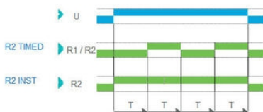
Function D - Symmetrical flashing (OFF Start)
