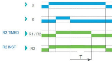
Function C - Off-Delay (Delay on break)
