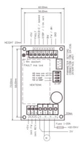
Molex connector options with dashed line 3-pin molex 22-27-2031 4-pin molex 10-08-5041 7-pin molex 22-27-2071
