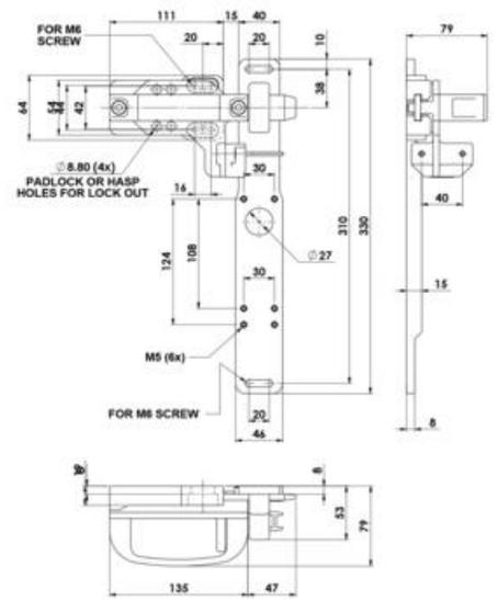
Handle GBZ with Rear Lever and Spring Loaded Catch
