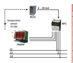
Control of a three-phase heater.
