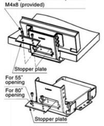
\*Opening angle can be limited to 55° or 80° with the included stopper plate.
