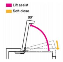
Opening angle can be limited to 55° or 80° with the included stopper plate.
