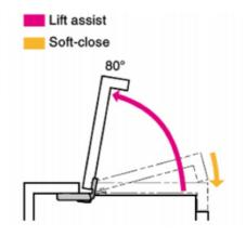
Opening angle can be limited to 55° or 80° with the included stopper plate.
