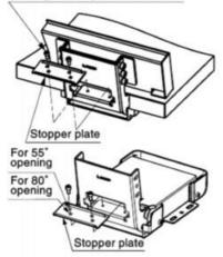
\*Opening angle can be limited to 55° or 80° with the included stopper plate.
