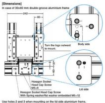
Use holes 2 and 3 when mounting on the lid side aluminium fran and holes 1 and 3 on the body side aluminium frame.
