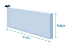
Installation height from 100 cm to 250 cm (from Reference Plane). Width: -5cm, + 5cm (fixed). Max length: up to 4m.
